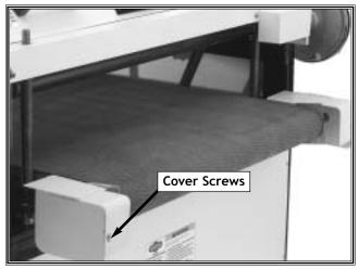
Figure 40. Infeed-conveyor safety covers.
